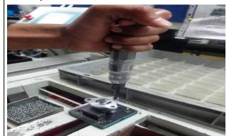
**COUNTERMEASURE-** To provided New eclectic tool for screw tightening.
